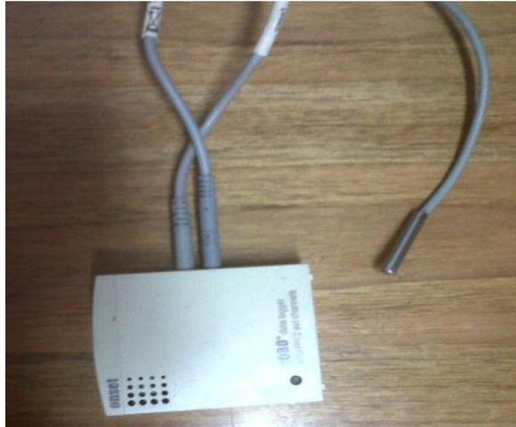
Figura 10 HOBO U12 Temp / HR /Luz / Externa Data Logger
