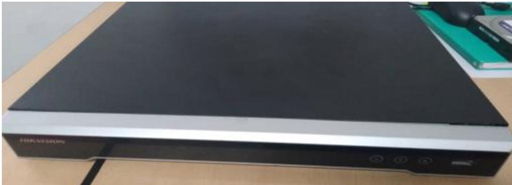
Imagen 5. Network video recorder (NVR).
